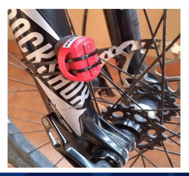
The transponder must be secured to the front fork of the bike using the provided plastic ties.
