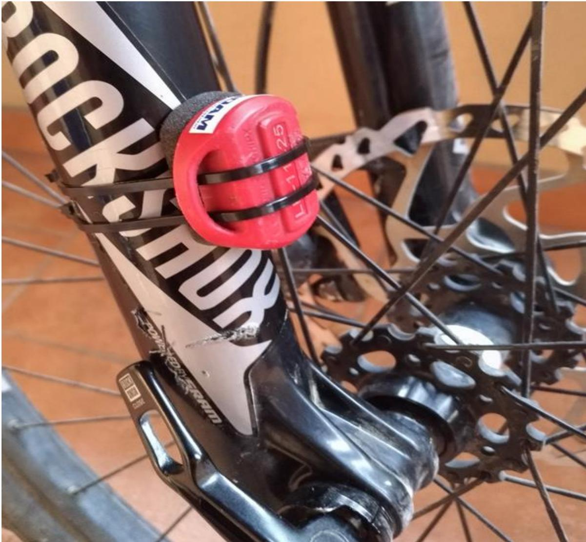
The transponder must be secured to the front fork of the bike using the provided plastic ties.
